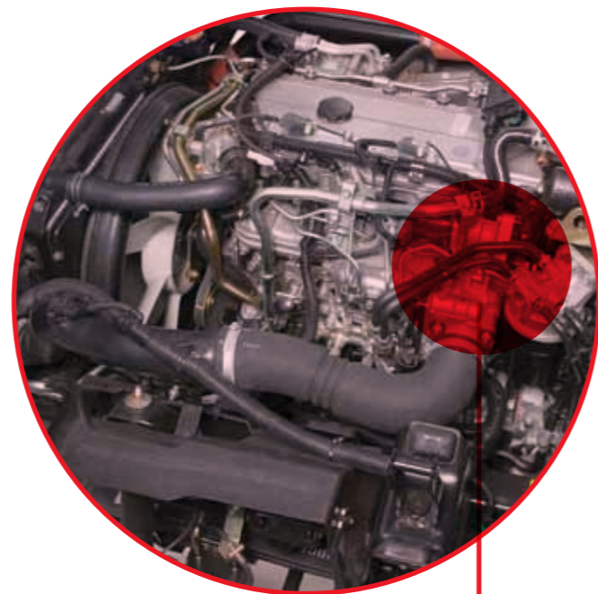
Exhaust Gas Recirculation (EGR) for the latest Euro emissions standard.
